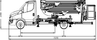
Max Working Height: 20m Max Horizontal Outreach: 10.7m
