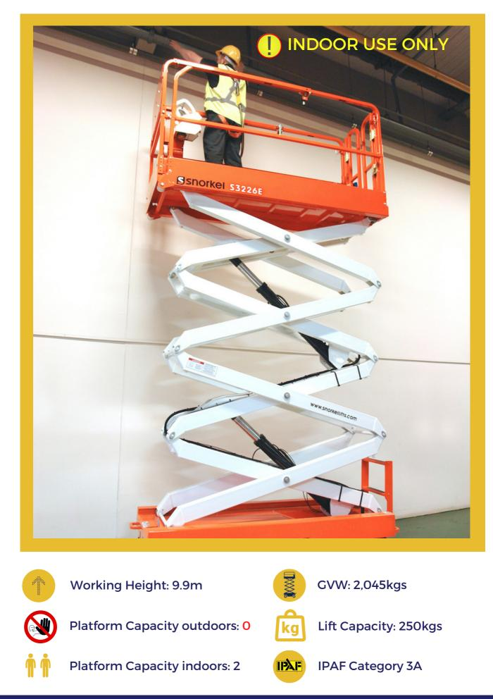
The Snorkel S3226E is a self-propelled electric scissor lift, with a working height of 9.9m. This is an '**Indoor Only**' rated scissor lift. It is battery powered, which offers quiet electric operation. With a maximum capacity of 250kgs, they are a perfect choice for both construction and industrial indoor maintenance work.
