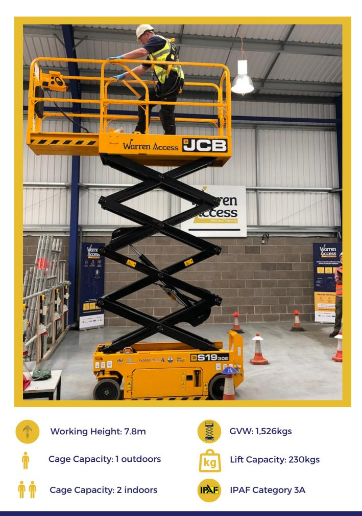
The JCB S1930E has 7.8m working height and is very popular for electric for work such as; construction fit-outs, maintenance tasks in factories, retail environments, warehouses and public buildings. These slab scissor lifts are lightweight, easy to manoeuvre and compact with zero inside turning radius.
