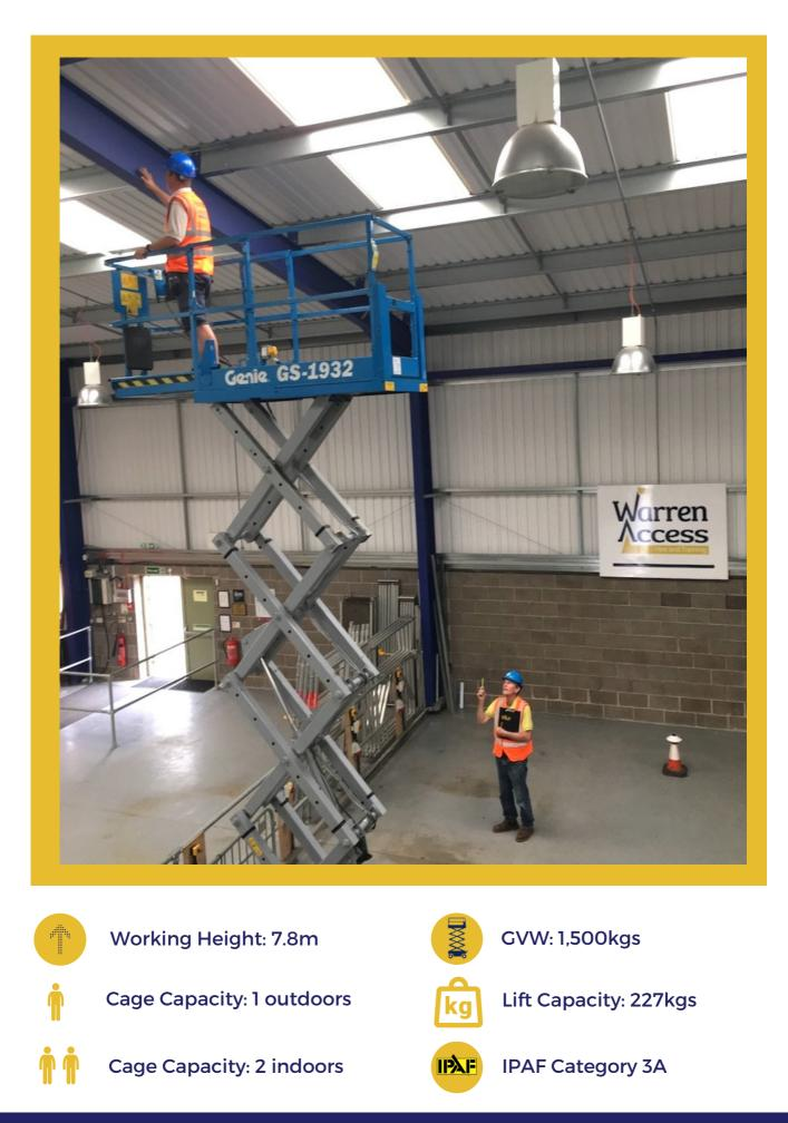
Genie slab scissor lifts can be used indoors or outdoors and offer quiet electric operation. The GS1932 has a working height of 7.8m and is designed for use on firm, level surfaces. They are an ideal tool if you are looking for electric scissor lift hire for indoor construction work, maintenance and installation work.
