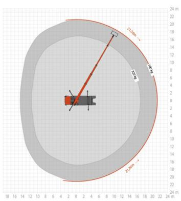
Max Working Height: 33m Max Horizontal Outreach: 21.2m Max Cage Floor Height: 31.0m Max Safe Working Load: 320kg Max Persons in Cage: 3 Max GVW: 7500kg
