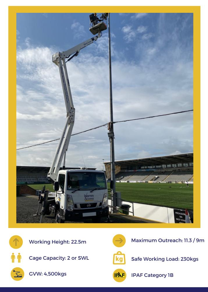
The versatile PNT230 has a working height of 22.5m and up to 11.3m horizontal outreach . It has zero tail-swing and is mounted on a compact 4.5t GVW truck. The dual pantograph boom allows work vertically up a structure with the operation of just a single control.
