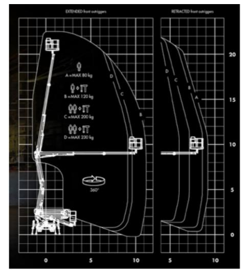
Max Working Height: 22.5m Max Horizontal Outreach: 11.3 / 9m Max Cage Floor Height: 20.5m Max Safe Working Load: 230kgs Max Persons in Cage: 2 Max GVW: 4,500kgs Cage Dimensions: 1.4 x 0.7m Travelling Machine Length: 6.4m Travelling Max Height: 2.5m Travelling Machine Width: 2.4m Working Machine Width: 2.6/2.4m Wheelbase: 2.9m
