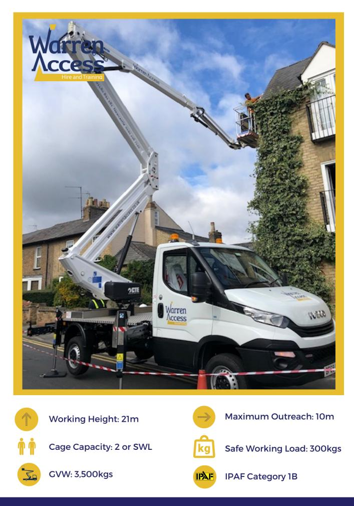
The CTE 21.3JHL is easy to use, with simple and intuitive controls and compact for easy handling. This is the first semi variable Zed21.3JHL mounted on the Iveco Daily. It boasts 10m of unrestricted outreach with 300kgs basket capacity.
