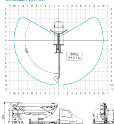
Cage Dimensions: 1.4 x 0.7 x 1.1m Travelling Machine Length: 7.48m Travelling Max Height: 2.8m Travelling Machine Width: 2.25m Working Machine Width: 4m Wheelbase: 3.75m
