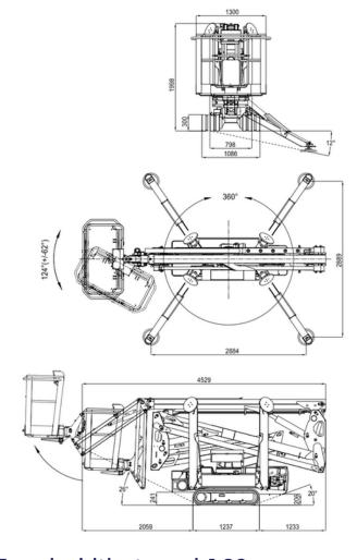
Travel width stowed: 1.09m Travel length stowed: 4.52m Travel height stowed: 2.0m Minimum travel width with cage removed: 0.80m
