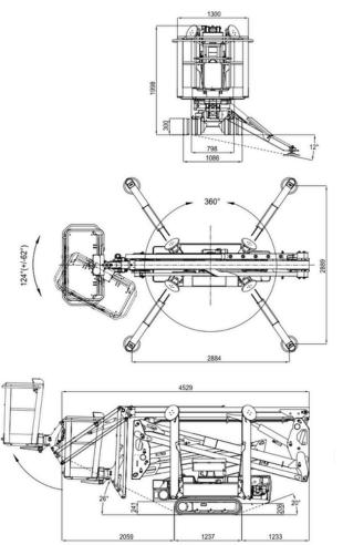
Travel width stowed: 1.09m Travel length stowed: 4.52m Travel height stowed: 2.0m Minimum travel width with cage removed: 0.80m Weight: 2,230kg Power source: Diesel / 110V mains
