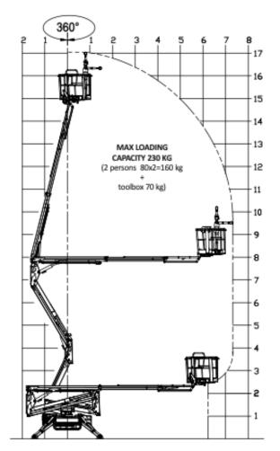
Max Working Height: 17.1m Max Horizontal Outreach: 7.5m Max platform capacity / occupants: 230kg / 2 persons Outreach at max. SWL: 7.5m Max lateral slope when travelling: 16 degrees
