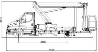
Max Working Height: 18m Max Horizontal Outreach: 13m Max Cage Floor Height: 15.5m Max Safe Working Load: 230kg
